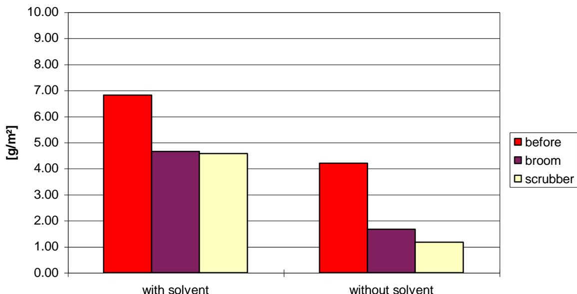
Figure 2: Dust surface concentration at beginning of duct before and after cleaning with broom and scrubber
