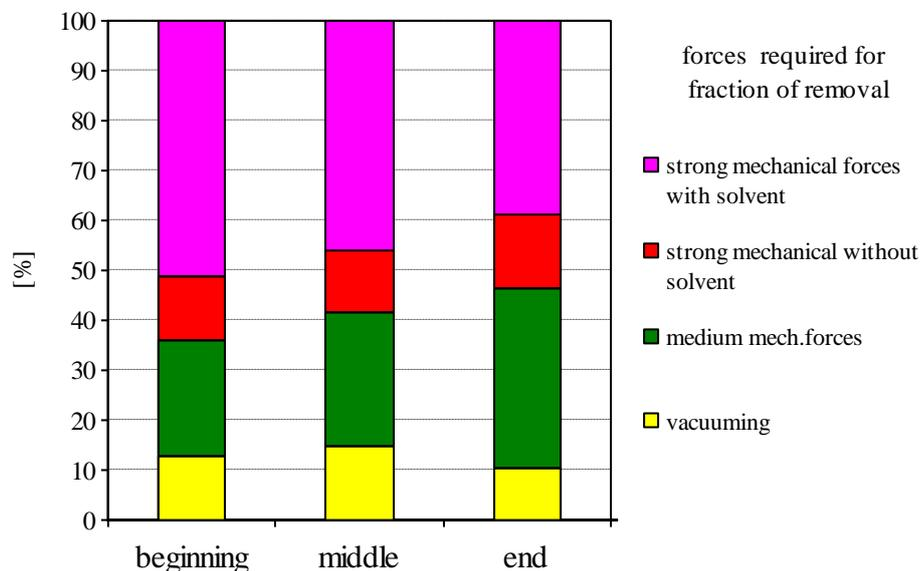
**Figure 1: Forces required to loosen dust from duct surface [%] at different locations of ventilation ducts (mean of 11 ducts), (Küchen, 1998).**
