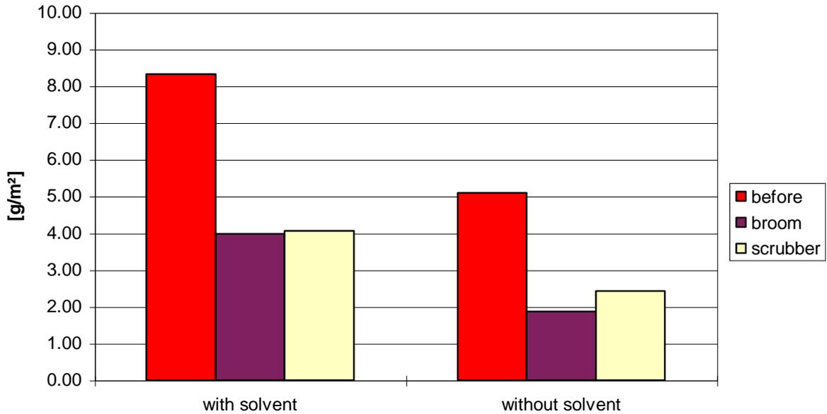
**Figure 3: Dust surface concentration at end of duct before and after cleaning with broom and scrubber**
