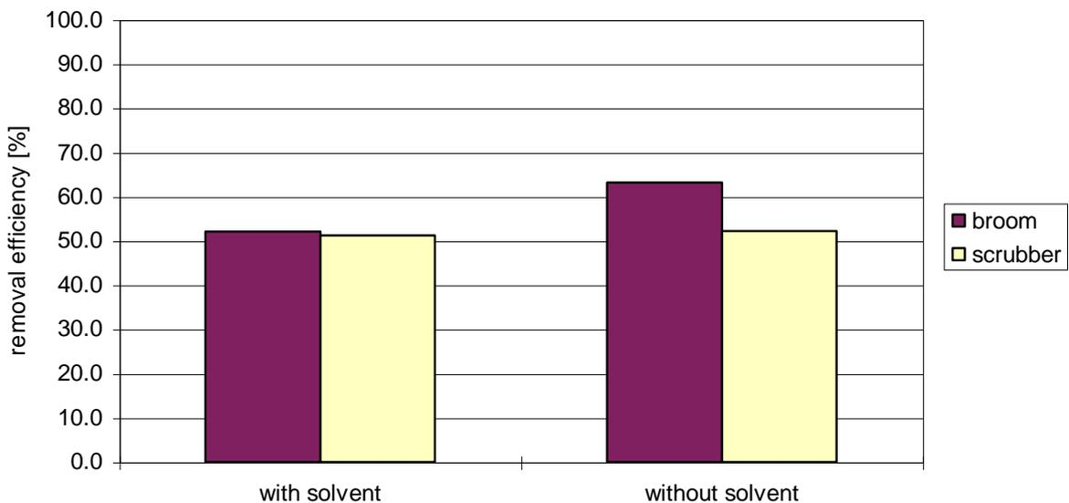
**Figure 6: Reduction of the dust concentrations by mechanical cleaning determined without solvent and with solvent [%] at end of duct**
