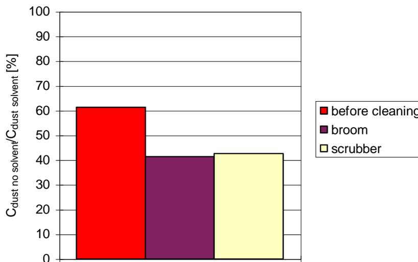
**Figure 4: Ratio of the dust concentrations determined without solvent and with solvent [%]**
