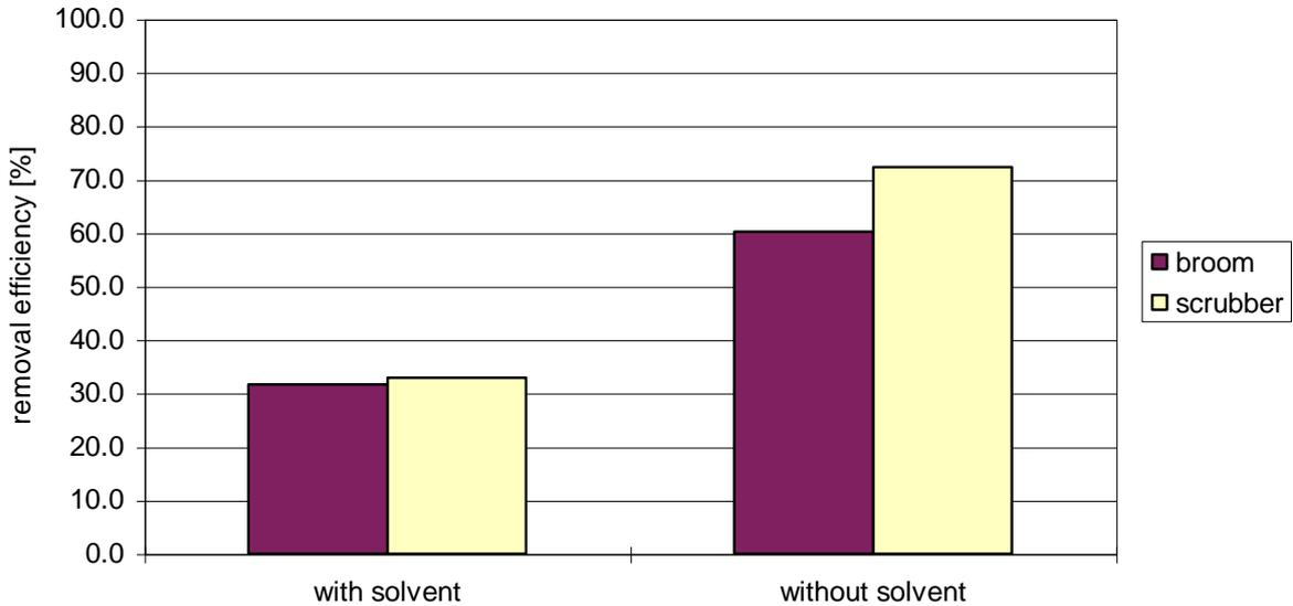
**Figure 5: Reduction of the dust concentrations by mechanical cleaning determined without solvent and with solvent [%] at beginning of duct**
